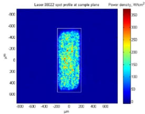
**Figure 3** – Intensity profile of Innovative Photonics Inc. “Stub laser” utilizing proprietary mode-mixing waveguide.
