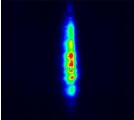
**Figure 1** – Non-uniform far-field intensity profile of conventional multimode laser showing intensity “hot spots”
