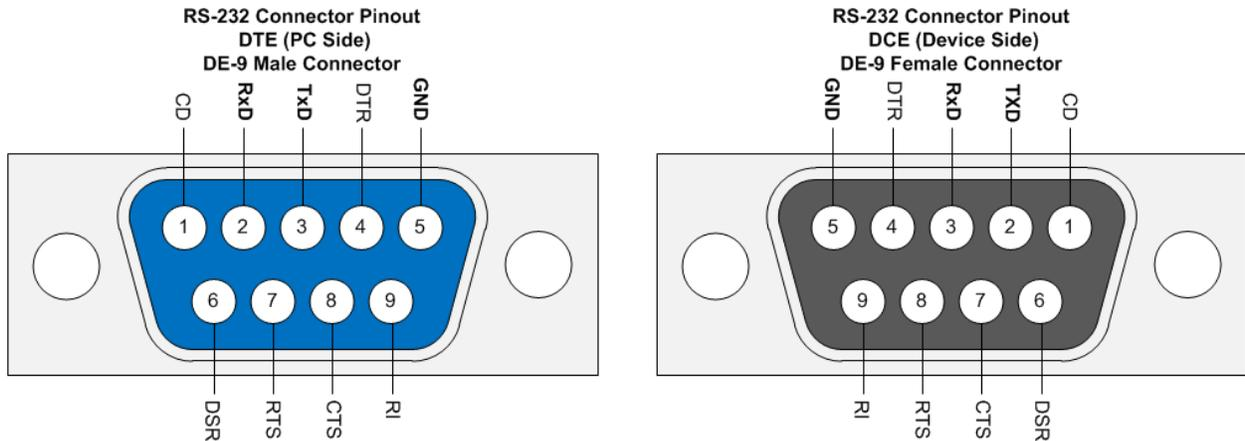
The Female DE-9 connector is the mirror image of the Male DE-9 connector. These diagrams show the connectors face-on.
