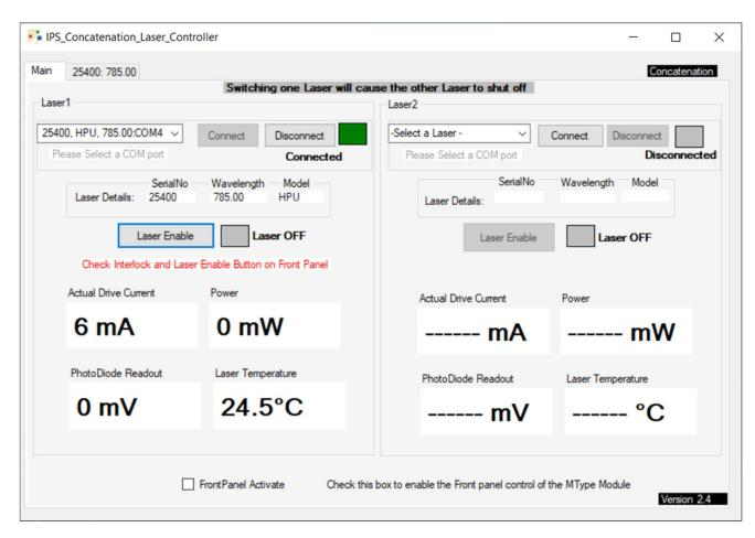
III. You will only be able to turn one laser on at a time. Clicking the "Laser Enable" button of the desired wavelength will toggle the laser on state from the current wavelength to the new wavelength. (If both lasers need to be operations concurrently contact IPS for instructions.)
