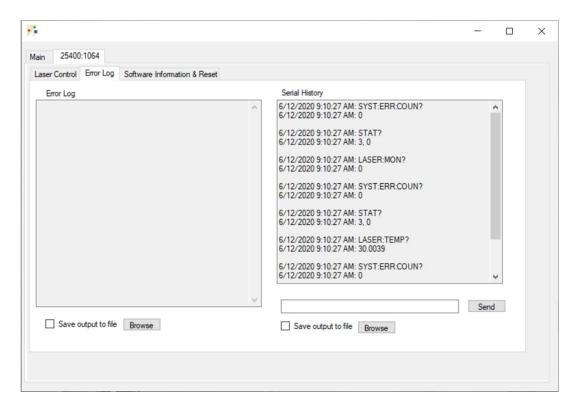
III. The "Module Operation Guide" may contain additional commands that are not included in this GUI. To utilize these commands, enter the command string in the field below "Serial History" and hit SEND. You can also use this field to test command codes when programming your own laser control software.
